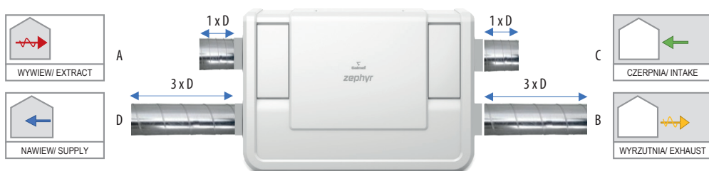
Fig. 12. Air duct length
